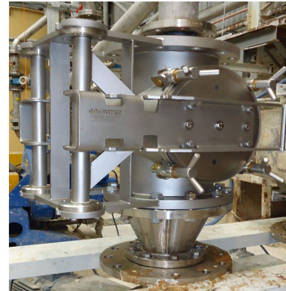
A magnetic separator in operation
